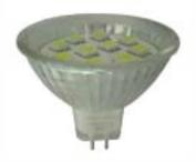
LED MR16 10 5050 SMT LEDs. GX5.3 Base. 12 volts AC/DC. Available in white only. Operates cool to the touch lasts upto 50,000 hours. Aproximate light output 130 lumens. This product measures approximately 1.90 inches by 1.95 inches.
