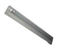
500 Lumen output. 145 forward firing LEDs and only uses 8 watts of power. 120 VAC. 4 Foot long. Interlink able T5 Tube lights. Has socket for input power and output Interlink able connection. The actual tube size without fixture is .60in x 48in and with the fixture its .90inx 48in x 1.83in. Inter connect cable is sold separately.
